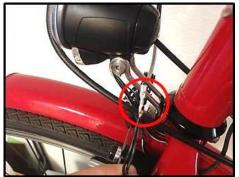
5. Pull the shrink tubing over the flat-plug shoes and, using a heat source (hot air gun or lighter), heat the tubing material so it contracts.
